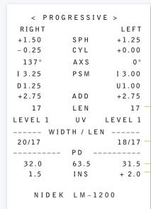
Printout sample in measurement of progressive power lens(es)
