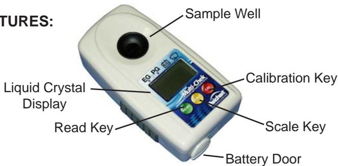
Using a Multi-Chek to test freeze point following the American Society for Testing & Materials (ASTM) Standard Practice D3321 provides results that are precise to  $\pm 0.5^{\circ}\text{F}$  ( $\pm 0.3^{\circ}\text{C}$ ) reading a 50 vol % aqueous solution of ethylene glycol. By comparison, a hydrometer is only precise to  $\pm 8.0^{\circ}\text{F}$  ( $\pm 4.44^{\circ}\text{C}$ ).
