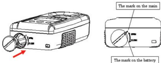
2. Align small mark found on the battery cover with mark found on the instrument body and insert cover as shown above.
