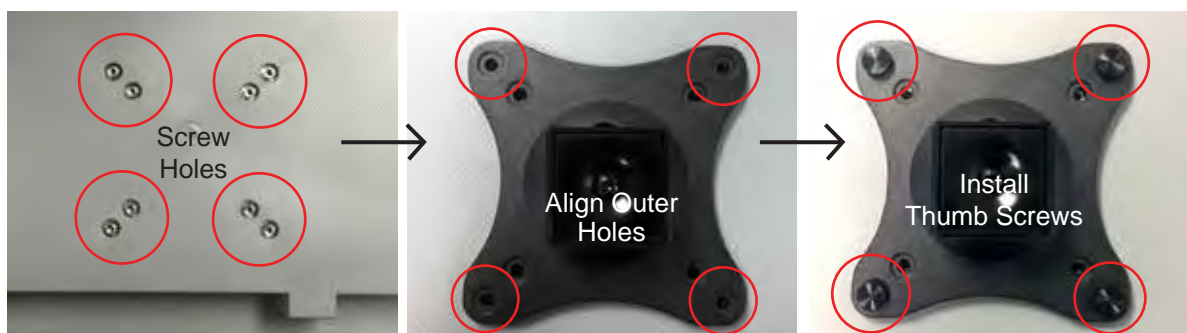
Figure SU-10 Align Holes and Attach Mount
