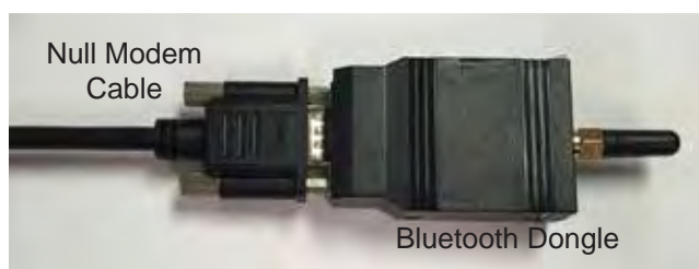
Figure SU-21 Connect Dongle to Cable
