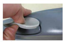
Figure CL-3. Remove Forehead Rest Pad
