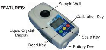
Using a EG-Chek to test freeze points following the American Society for Testing & Materials (ASTM) Standard Practice D3321 provides results that are precise to  $\pm 1.0^{\circ}$ F ( $\pm 0.6^{\circ}$ C) reading a 50 vol % aqueous solution of ethylene glycol. By comparison, a hydrometer is only precise to  $\pm 8.0^{\circ}$ F ( $\pm 4.4^{\circ}$ C).
