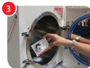
3 Open the door and spread the contents of a packet of Chamber Brite™ in a straight even line along the bottom of a **cold** chamber, from back to front.
