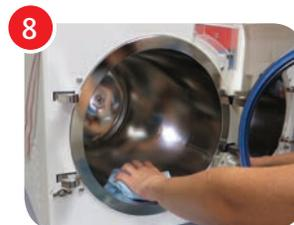
8 Wipe the interior of the chamber with a damp cloth or sponge. Clean the water sensor in the rear of the chamber with a damp cloth or sponge. Cleaning the dirt off the sides of the sensor is more important than the tip. (see sec. 12.6). The unit is now ready to sterilize.
