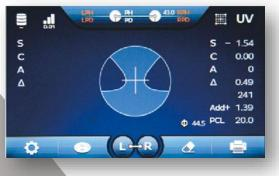
Measurement of PD, PH and PCL (Progressive Channel Length).
